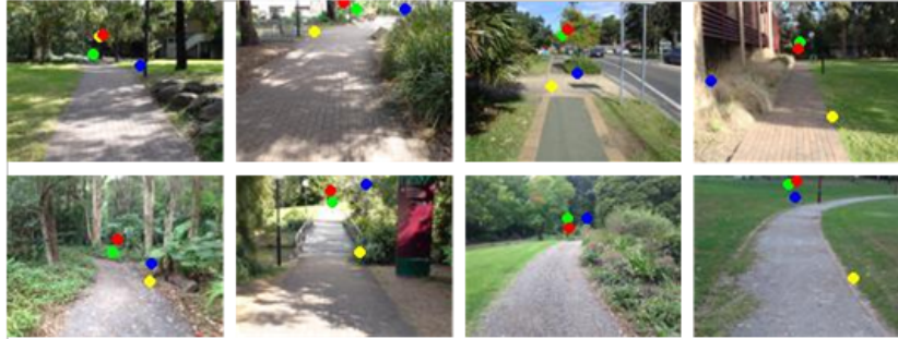
Fig. 7. Visual results of vanishing point (VP) detection: red dot is the ground-truth VP; green dot is the VP detected by the proposed method; yellow dot is the VP detected by Hough-based method [4]; blue dot is the VP detected by Gabor-based method in [2]. See electronic color image.
