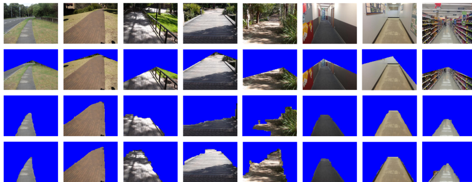
Fig. 8. Visual results of different methods for pedestrian lane detection. Row 1: input images. Row 2: pedestrian lanes detected by the method in [2]. Row 3: pedestrian lanes detected by the proposed method using the RGB color space. Row 4: pedestrian lanes detected by the proposed method using the IIS color space.
